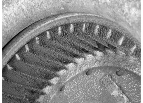
This reduced air flow decreases system performance. As little as 1/10 of an inch of dust on your blower blades can have a dramatic impact on system performance, efficiency, and longevity.
