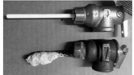
This photo compares a new T&P Valve (above) with one with sediment buildup insulating the temperature probe.
